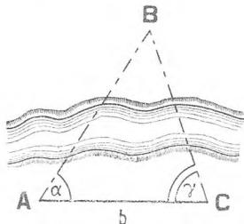
$$\frac{AB}{\sin \gamma} = \frac{b}{\sin (180^\circ - \alpha - \gamma)} = \frac{b}{\sin (\alpha + \gamma)},$$
